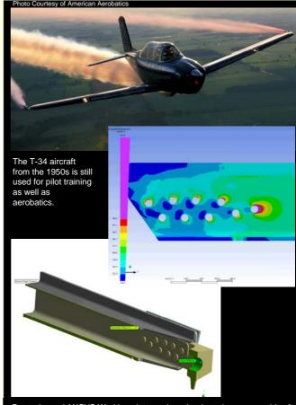
Raetech used ANSYS Workbench to analyze the riveted spar assembly of a T-34 aircraft under a range of loading conditions (lower left). The simulation accurately determined stresses and fatigue life (upper right), proving an adequate design for the aircraft when flown within the prescribed limits.
